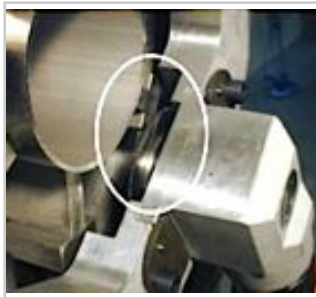
Optimized blade-jaws distance Limits vibration and tube distortion
