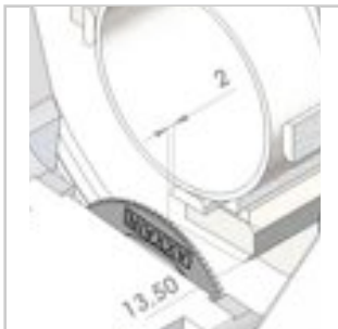
Blade-jaw distance of 2/13.5 mm. Limits vibration and tube distortion
