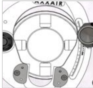
Concentric clamping with 4 jaws in stainless steel , standard, to eliminate tube distortion
