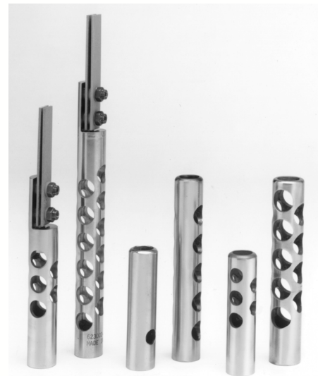
Typical Probe Element Shields. Coupon holding on the left, High Velocity in the Middle, Standard on the right.
