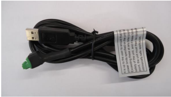
High speed transfer data TTL cable (fig. 11).
