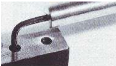
A 5/64" UNBRAKO key will twist up to 180° without weakening.
