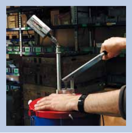
simalube can be filled as well as refilled by using a standard barrel pump that is typically used to fill grease guns.
